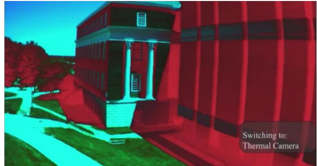
Figure 1: We developed five automated thermography scenarios inspired by the research literature ( e.g. , [6,10,35,41]) to help elicit reactions to envisioned automated solutions. Above, a screen capture from our unmanned aerial vehicle (UAV) design probe. See supplementary video.
