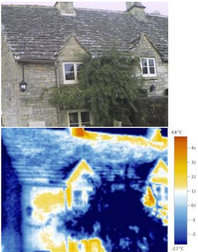
**Figure 1: Energy auditors use thermal imagery cameras to find poor insulation and air leakage. The thermal image above taken in the winter shows heat leaking out of the rooftop and windows (from an energy assessment report [8]).**
