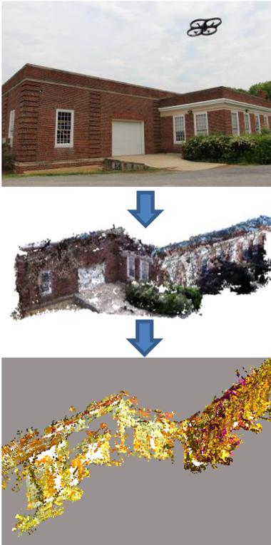
**Figure 6: Example of partial 3D-reconstruction using UAV and data from our thermal camera.**
