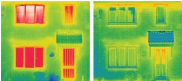
**Figure 2: A building façade before a renovation (left) and after (right). The thermal imagery highlights significant improvements in heat loss through the installation of energy-efficient windows and doors (from [7]).**
