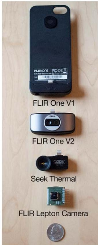
**Figure 2:** Smartphone-based thermal cameras (top to bottom): FLIR One (version 1), FLIR One (version 2), Seek Thermal. The fourth item is a FLIR Lepton Camera and connective housing that can be used for electronics projects (and hackathons).
