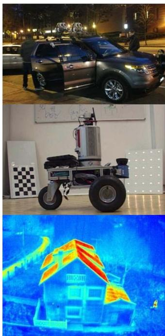
**Figure 4:** Examples of thermal data collection techniques from research literature and in industry: (a) Essess Inc.'s Google Street View like cars with mounted thermal cameras [12]; (b) Irma3D indoor thermal mapper robot [15]; (c) residential data from a UAV with a mounted thermal camera [11].
