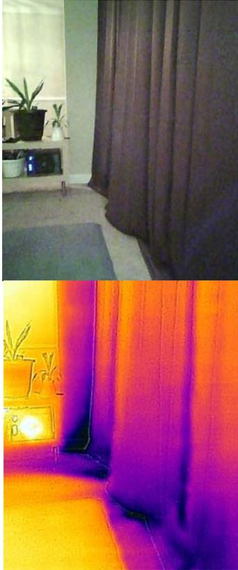
**Figure 6:** A participant in our pilot study described using a thermal camera to measure temperature exchange in her apartment resulting from the floor-to-ceiling windows (behind the curtains). The pilot participant took photographs over several hours and deduced that the rate of thermal exchange increased as a function of the difference between the internal and external temperatures; this experiment was designed to confirm a previous comfort concern.
