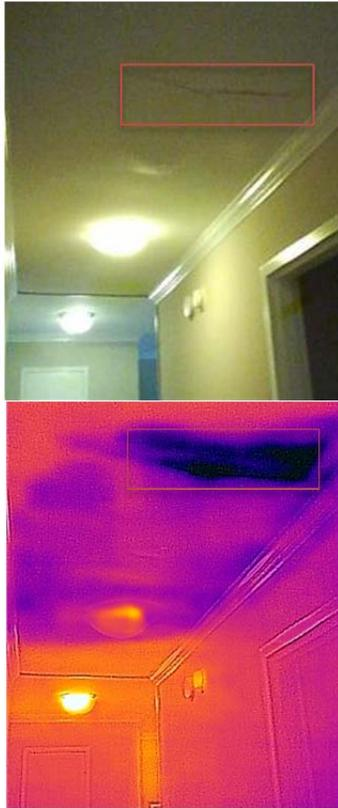
**Figure 3:** A participant in our pilot study noticed a small drip in the ceiling of her apartment and used her thermal camera to survey the extent of the moisture damage. To the unassisted eye (top), the leak appeared to impact only a small section of the ceiling where there was a visible crack; however, the thermal photograph (bottom) shows that the damage extended throughout the hallway. This photo (and others) was used to report the issue to maintenance personnel.
