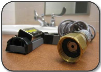
**Figure 8.** An early version of the HydroSense water sensor, capable of sensing water activities down to the fixture level (e.g., toilet, shower, etc.) from a single installation point.
