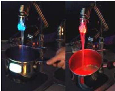
**Figure 2.** HCI and UbiComp researchers are well positioned to use their expertise in design, information perception, and sensor systems to create a new generation of feedback technology such as HeatSink, a water temperature feedback device by Arroyo et al., 2005.
