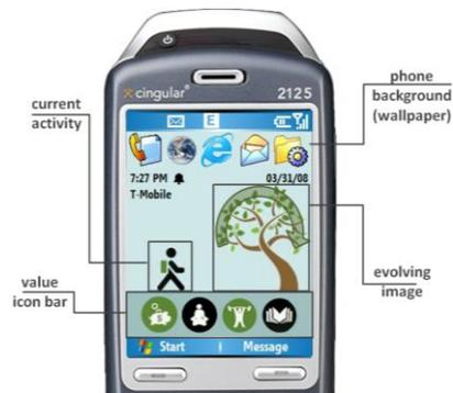
**Figure 4.** The UbiGreen Transportation Display automatically updates the background display of a user's mobile phone based on green transportation usage. The interface serves as a personal ambient display, visible whenever the user picks up the phone for everyday purposes (e.g., to make a phone call or send a txt message).
