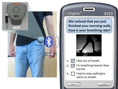
**Figure 3.** MyExperience allows researchers to trigger self-report surveys at automatically sensed points of interest. In the above scenario, a question about breathing rate is asked after an activity-inference sensor detects the end of a morning walk.
