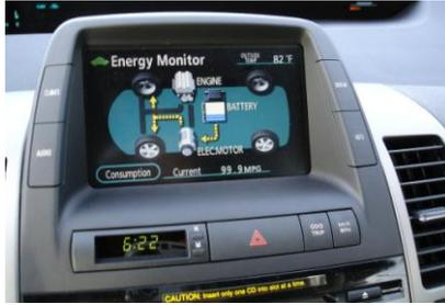
**Figure 1.** The Toyota Prius introduced perhaps the canonical example of an effective energy feedback display, providing real-time information about combustion engine vs. electric motor usage enabling people to drive more efficiently as a result.
