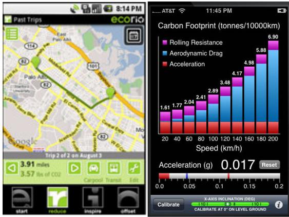
**Figure 4. (left) ecorio runs in the background of the phone and keeps track of car and bus trips via GPS to calculate carbon impact. (right) greenMeter uses the mobile phone's internal accelerometer to measure forward acceleration and compute fuel economy and carbon footprints.**
