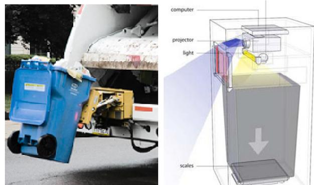
**Figure 6. (left) RecycleBank automatically tracks household recycling using RFID and electronic scales. (right) JetSam is a prototype trash tracking system that snaps pictures and weighs trash as its deposited.**
