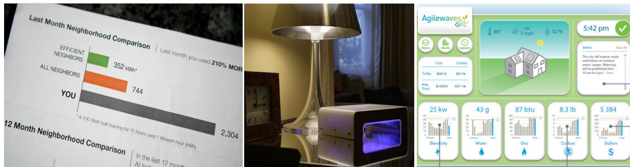
Figure 2. (from left-to-right) The Positive Energy paper bill with neighborhood comparisons. The Wattson ambient display which glows according to energy consumption level. The AgileWaves internet portal for the home displays energy usage information for gas, water, and electricity and allows the user to “drill-down” to finer levels of detail.
