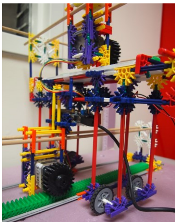
Figure 2. The AtmoSPHERE prototype system consists of four pairs of 3D printed gears and tracks, two stepper motors, one super magnet marble inside a sand box, and a Kinect that can detect the room occupants' noise levels as well as track their movement.
